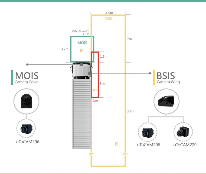
BSIS: Through the front and rear cameras in the camera wing, pedestrians and cyclists can be detected in the vehicle's side blind area in different scenarios.
